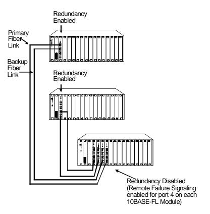
Figure 2-11. Total Backbone Fault-Tolerant Configuration
